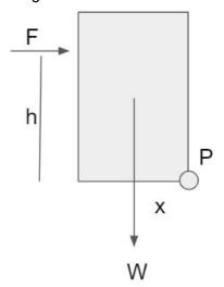
The moment about P is the component of Fh perpendicular to P minus the component of Wx perpendicular to P, so the box will rotate clockwise about P if F > Wx/h. The wider the base of an object, the more stable it is.
